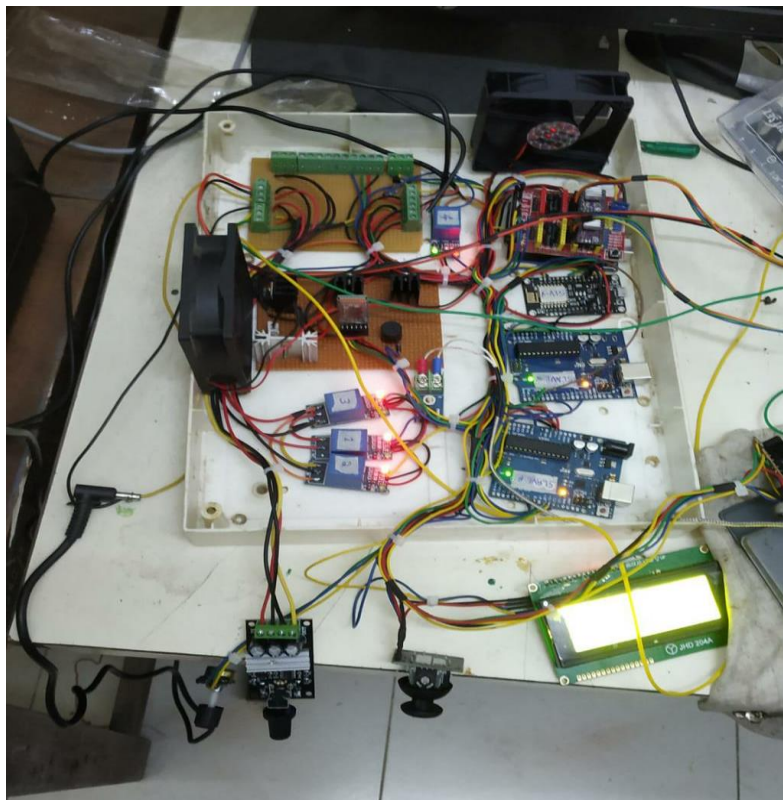
Fig 4.10 fabricated circuit for both motion control and ECDC process
