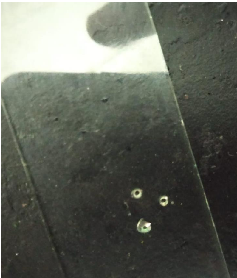
Fig 5.1 Holes machined on glass workpiece of 2 mm thickness at a federate of 3 mm/min
