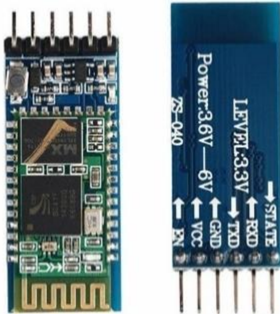
Fig 2.8 hc05 Bluetooth module
