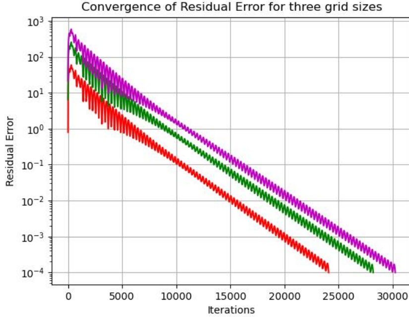
Figure 29: Convergence for Re = 100 for the artificial compressibility method.
